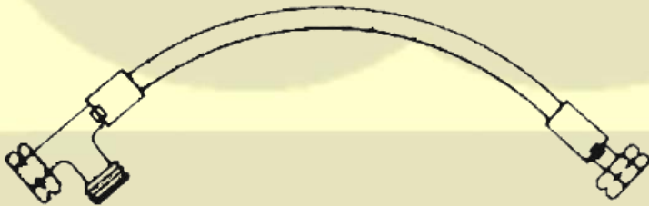
321 Flexible Two Bottle Connection F.E.C.V. X F.E.C.V. With 1 M.E.C.V. nipple one end.
